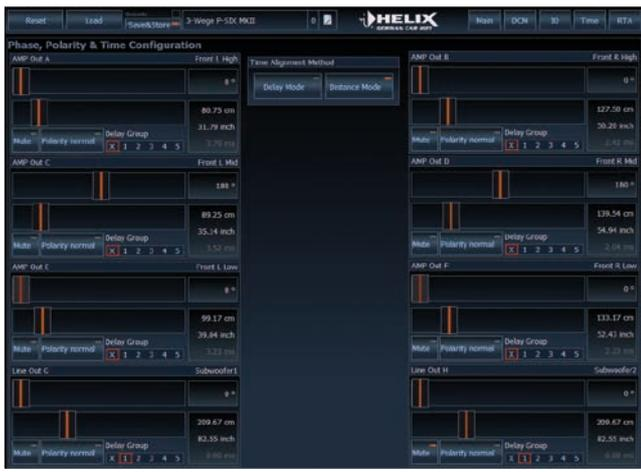
The TIME page gives a very simple overview of all time alignment and phase adjustments of every channel at a glance. It offers two adjustment modes; the delay mode allows entering direct delay values whereas the distance mode enables inserting the measured distances to each speaker and the DSP PC-Tool automatically calculates the necessary time delay for each channel.
